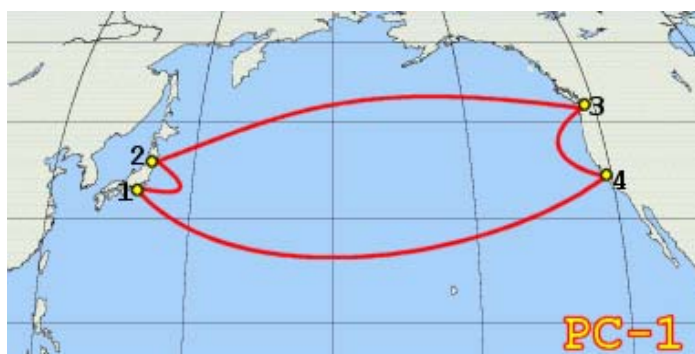
Figure 1: Diagram of the PC-1 Network Landing points: In Japan: Shima, Ajigaura In the US: Harbour Pointe, Washington; Grover Beach, California
